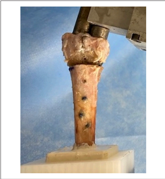
Figure 3. Application of axial load with 60/40 distribution (lunate/scaphoid facets respectively) via an angled vise.
